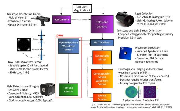
Figure 2. HiCIBaS systems schematic of the complete mission concept including the telescope and star tracker, the Low-Order WaveFront Sensor (LOWFS) and the DM arm that includes the deformable mirror, coronagraph and science camera [7].
