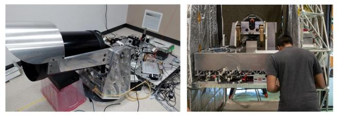
Figure 1. HiCIBaS payload in the laboratory (left) and integrated in the gondola (right)
